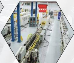
PVC tubing is extruded in our own facility to maintain a consistent formulated standard for UV stabilization, strength, and wear resistance.
