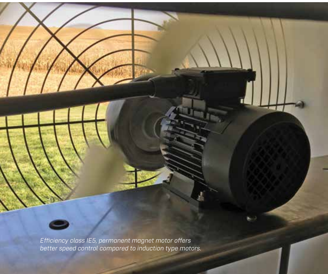
The Optidrive provides precise motor control and energy savings using the custom programs for each Commander fan.
